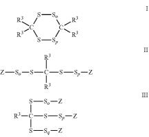
wherein each  $R^3$  is independently H or a  $C_1$ - $C_{20}$  organic moiety, o, p and q are each independently an integer of 1 or more, and each Z is independently a  $C_1$ - $C_{20}$  organic moiety, Li, Na, quaternary ammonium, or quaternary phosphonium. Examples of such organosulfur species include 1,2,4,5tetrathiane (formula I,  $R^3$ —H, o=p=1), tetramethyl-1,2,4,5tetrathiane (formula I,  $R^3$ —CH<sub>3</sub>, o=p=1), and oligo or polymeric species thereof.
