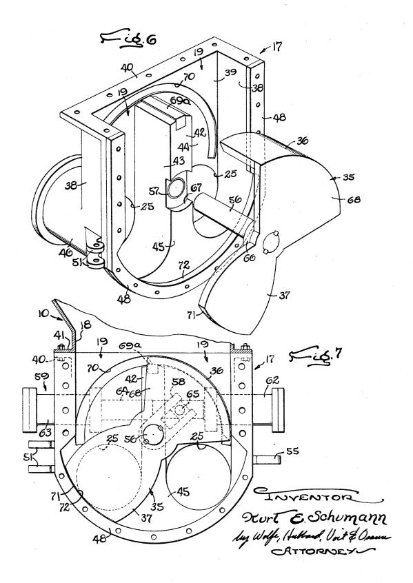
CONCRETE PUMPING APPARATUS
