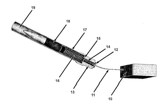
(57) Abstract: The invention comprises a device and method for firing firearm ammunition using an EMP generator (10). The device can be incorporated into or used with firearms of a variety of sizes and configurations to provide precise control of firing and improved range and safety. The device and method can be applied to conventional mechanical primer ammunition or used without the need for a primer, particularly in field artillery, aircraft, and watercraft.
