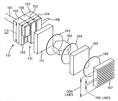
timally close spacing to achieve the desired result. In one embodiment, the laser diode pumps are directly modulated by the video signal, while in another embodiment the microlaser outputs are modulated utilizing a spatial light modulator array.
