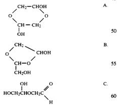
In addition, glycol aldehyde forms acetals and hemiacetals with methanol, and, if present, ethylene glycol. Acetals in particular are resistant to hydrogenation and 65 should preferably be hydrolyzed to the free aldehyde so that efficient reduction to ethylene glycol can be effected.
