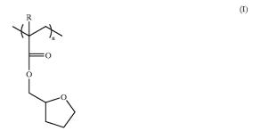
wherein R is selected from the group consisting of —H and — $C_1$ — $C_6$  alkyls and n is an integer greater than or equal to 1; and an oxidation catalyst. The oxygen scavenging polymer can be used to form an oxygen scavenging packaging article.
