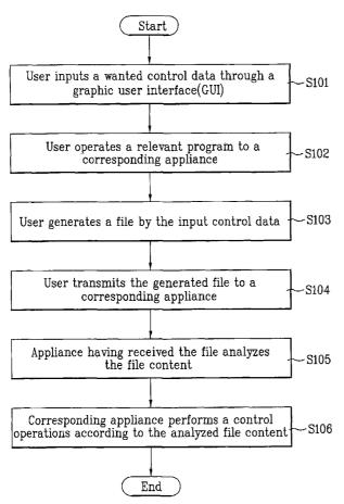
**(57) Abstract:** A method for controlling a home network system is disclosed. The method includes a step for inputting control data; a step for generating a file by the input control data; a step for transmitting the generated file to a corresponding appliance; and a step for performing a corresponding control function by analyzing the transmitted file.
