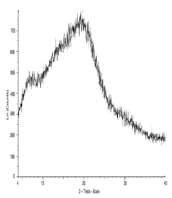
10/90 FP/DPS (3448-045) – File: 3448-045.raw – Type: 2Th alone – Start: 4.000° - End: 40.000° - Step: 0.040° - Step: time: 2 s – Temp: 25°C (Room) – Time Started: 15 s – 2-Theta: 4.000° - Theta 3.000 Operations: Import
