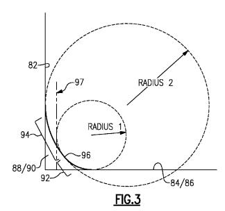
(57) Abstract: A guide vane has an airfoil and a platform at least at one end of the airfoil. A compound fillet blends the airfoil into the platform. The compound fillet has a first portion at a first radius of curvature adjacent to the platform, and a second portion at a second radius of curvature blending from the first portion into the airfoil. The second radius of curvature is different than the first radius of curvature.
