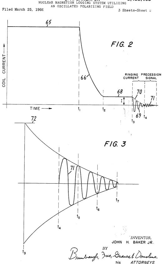
Dec. 9, 1969 J. H. BAKER, JR NUCLEAR MAGNETISM LOGGING SYSTEM UTILIZING AN OSCILLATED POLARIZING FIELD 3,483,465
