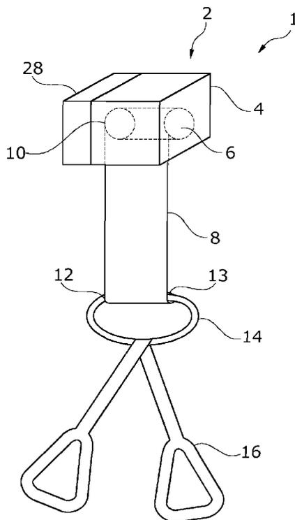
(57) Abstract: The invention relates to an exercise device comprising at least one elongate part whose length can be adjusted. At least one wind-up device is fixed to an object by means of fastening means and has a shaft for winding and unwinding the elongate part, a first end of said elongate part being fastened to the shaft. The exercise device further comprises a locking device for releasably immobilizing the elongate part in various positions relative to the wind-up device.
