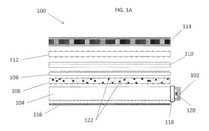
(57) Abstract: Disclosed herein are display systems comprising light-emitting diodes (LED&), suitably blue light LEDs, which demonstrate increased optical power output. In embodiments, the display systems include compositions comprising phosphors, including luminescem nanocrystals.
