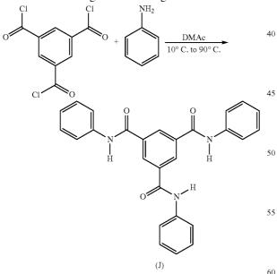
The experimental set up consists of a 2 L glass beaker equipped with a glass rod stirrer coupled with an overhead mechanical stirrer. Trimesoyl chloride (200 g) is dissolved in dimethyl acetamide ("DMAc") (1 L) and cooled by an ice 65 bath to 10-20° C. Aniline (421 g) is added drop wise to a stirred solution of the acid chloride over a period of 1.5 to 2
