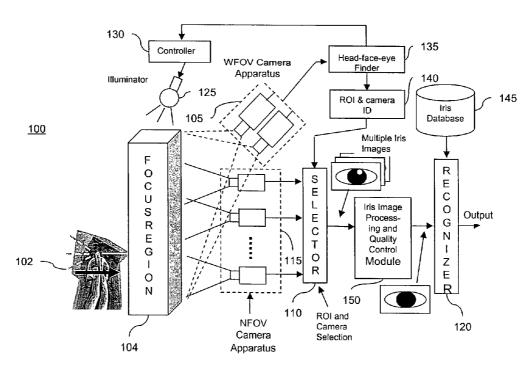
(57) **Abstract:** The method and apparatus for performing iris recognition from at least one image is disclosed. A plurality of cameras (105, 115) are used to capture a plurality of images where at least one of the images contains a region having at least a portion of an iris. At least one of the plurality of images is then processed to perform iris recognition (120, 145).
