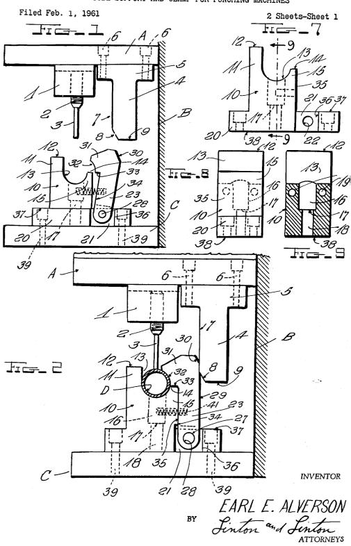
TUBE SUPPORT AND CLAMP FOR PUNCHING MACHINES
