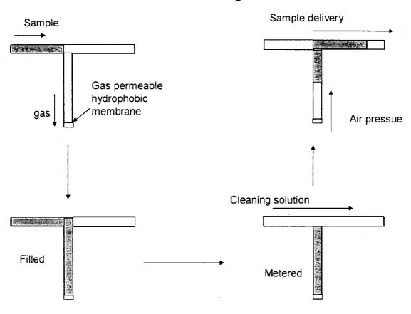
Air pressue Sample delivery Cleaning solution Conventional metering method Metered Gas permeable hydrophobic membrane Sample gas Filled
