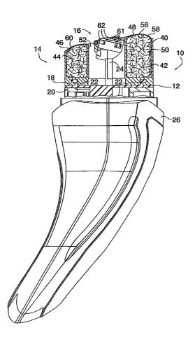
(57) Abstract: A shaving apparatus (10) is provided that is selectively attachable to a handle (26). The cartridge includes a razor cartridge (16) and a device for dispensing a non-solid shaving aid material. The shaving apparatus (10) attaches to the handle (26) in such a manner that a self-leveling mechanism (30) contained within the handle is not operable to adjust the movement of a first element relative to a second element.
