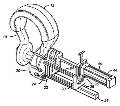
(57) Abstract: The present inventions relate generally to a shackle assembly and a method for installing and/or releasing the shackle assembly subsea. The shackle assembly of the present invention comprises first (20) and second (22) plates mounted on either side of a shackle body eyelet (14) and a shackle pin mounting assembly (26, 28, 30, 32, 34. and 36) for use in mounting a shackle pin (38) using a shackle pin pulling tool (44).
