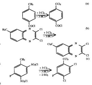
The process according to the invention is carried out at a temperature of 120°-240° C., preferably 160°-220° C. and at a pressure of 0.5-5 bar, preferably of 1-1.5 bar. The reaction times are dependent in a manner known to those skilled in the art on the size of the reaction batch, but in general are only approximately 25 to 85% of the time which is necessary without the catalysis according to the invention. 10
