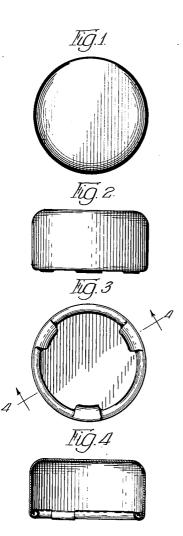
Fig. 1 is a top view of a closure cap for bottles or the like which embodies my new design;
