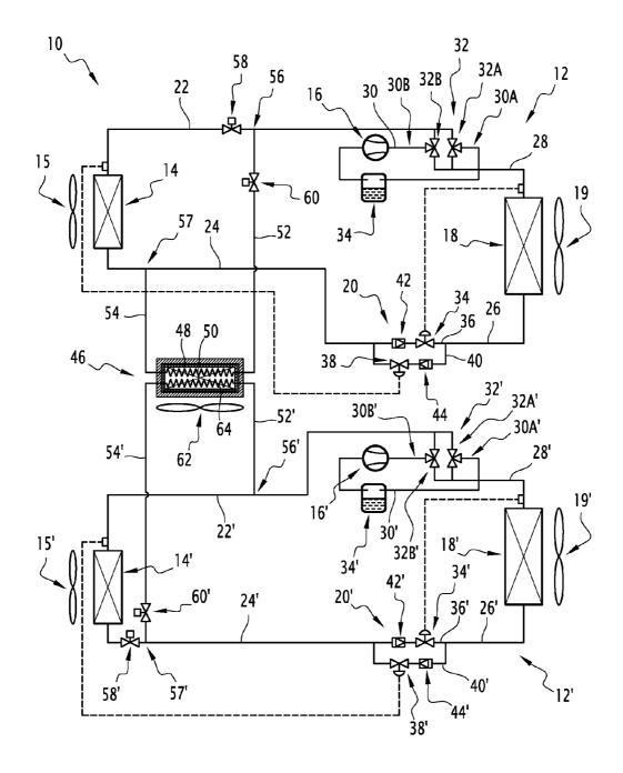
**[0001]** The present invention relates to an air conditioning device for a compartment, in particular for a railroad vehicle. **[0002]** A device is already known from the state of the art for air conditioning a compartment, comprising a heat pump circuit. Said heat pump circuit traditionally comprises a first heat exchanger with the air in the compartment, a compressor, a second heat exchanger with the outside air, and an expander, all arranged in series in a closed circuit to form a loop.
