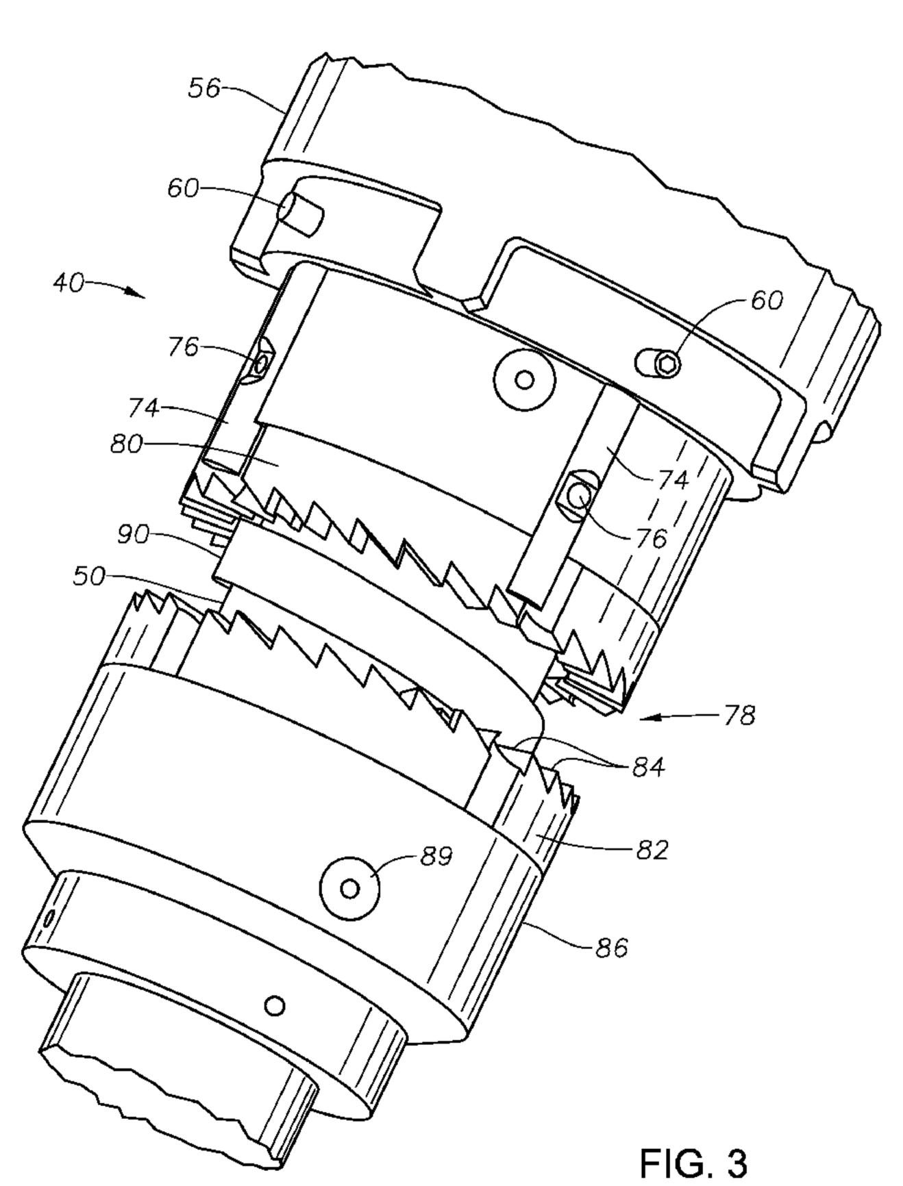
(57) Abstract: Devices and method for engaging a casing member for manipulation. A hydraulic torque locking mechanism is incorporated into a casing manipulation assembly. The hydraulic torque locking mechanism includes a clutch mechanism that is actuated using surface pump pressure from tool circulation.
