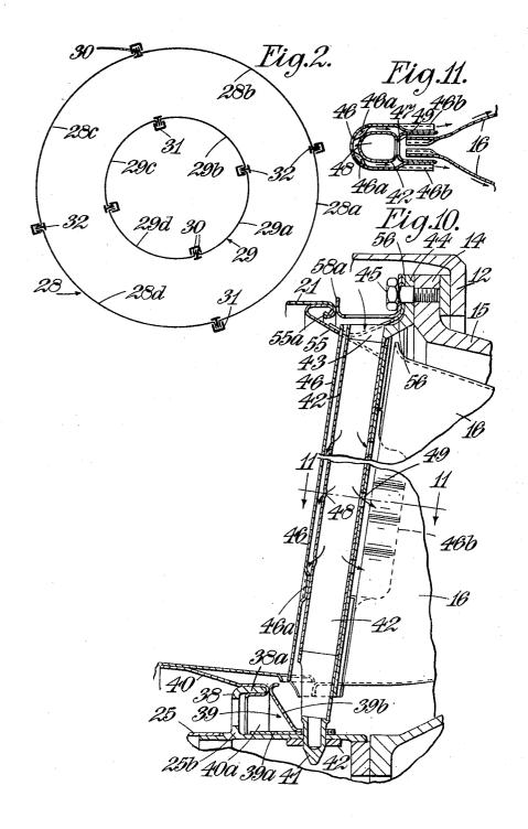
G. OULIANOFF ET AL FLAME TUBE STRUCTURE FOR COMBUSTION EQUIPMENT OF GAS-TURBINE ENGINES
