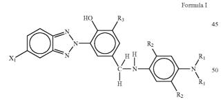
wherein  $R_1$  and  $R_2$  are  $C_1$  to  $C_8$  linear or branched alkyl;  $R_3$  is hydrogen, tert-butyl;  $X_1$  is select the group consisting of hydrogen, halogen, tert-butyl and  $C_1$  to  $C_{12}$  alkoxy, where the compound has antioxidant and antiozonant properties, and a process for the synthesis thereof.
