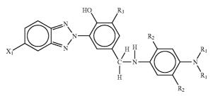
wherein  $R_1$  and  $R_2$  are  $C_1$  to  $C_8$  linear or branched alkyl;  $R_3$  is hydrogen, tert-butyl;  $X_1$  is select the group consisting of hydrogen, halogen, tert-butyl and  $C_1$  to  $C_{12}$  alkoxy.
