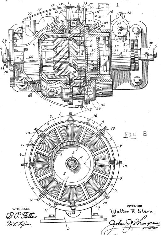
W. F. STERN. ROTARY GAS ENGINE. APPLICATION FILED APR. 29, 1911.
