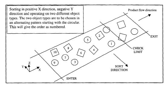
(57) Abstract: System for selection and transport of an object out of a plurality of objects in an operation area comprising a system for detection of objects present in the operation area and an industrial robot including a manipulator and an operating system having a computer memory for storing information on the objects present in the operation area.
