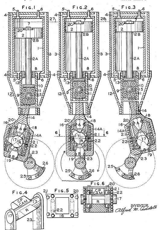
PRESSURE RETAINING MEANS FOR DOUBLE-ACTING PISTON ENGINES
