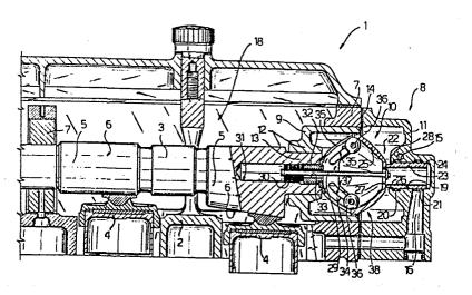
Device for regulating the axial position of a variable-profile camshaft, in particular for controlling the timing system on an engine.
