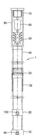
(57) Abstract: Apparatus and methods are provided for a cementing operation for use with a drilling with casing application. In one embodiment, an apparatus (1) is provided for stage cementing using a full opening stage tool (30). In another embodiment, an apparatus is provided for reverse cementing of the casing.
