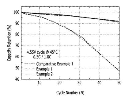
POSITIVE ELECTRODE ACTIVE MATERIAL PARTICLE INCLUDING CORE CONTAINING LITHIUM COBALT OXIDE AND SHELL CONTAINING COMPOSITE METAL OXIDE AND PREPARATION METHOD THEREOF
