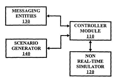
(57) Abstract: An embodiment of the invention generally relates to a method of real-time simulation. The method includes providing a continuous real-time clock (110) to a non real-time simulator (120) and synchronizing a simulation clock of the non real-time simulator with the continuous real-time clock on a continuous basis. The method also includes advancing the non real-time simulator to a first time based on the simulation clock reaching the first time.
