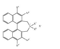
(wherein  $Ar^4$  and  $Ar^{4'}$ , each independently represents an optionally substituted phenyl group,  $R^7$  and  $R^8$ , each independently represents an aliphatic hydrocarbon group having 1 to 12 carbon atoms,  $R^9$  and  $R^{9'}$ , each independently represents a hydrogen atom, an aliphatic hydrocarbon group having 1 to 12 carbon atoms or an alkoxy group having 1 to 12 carbon atoms, and  $X^-$  represents a monovalent anion).
