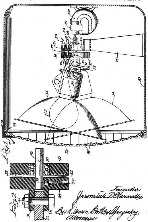
OSCILLATING WARNING LIGHT Filed Dec. 6, 1945 2 Sheets-Sheet 2
