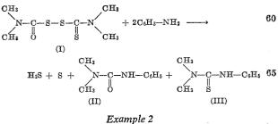
Tetramethylthiuram monosulfide (20 g., 0.1 mole) was slurried in 150 ml. toluene at room temperature (20° C.) with vigorous stirring. Nitrogen tetroxide (4.6 g., 0.05 mole) admixed with air was bubbled into the mixture. The solids slowly dissolved and when all of the 75
