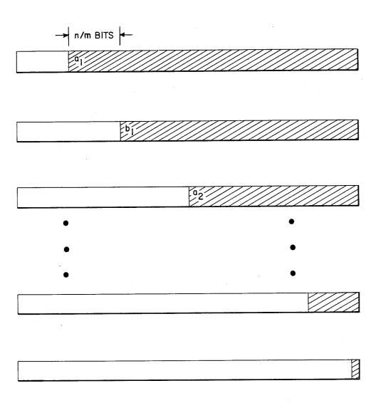
Fig.5 CONVOLUTIONAL INTERLEAVING
