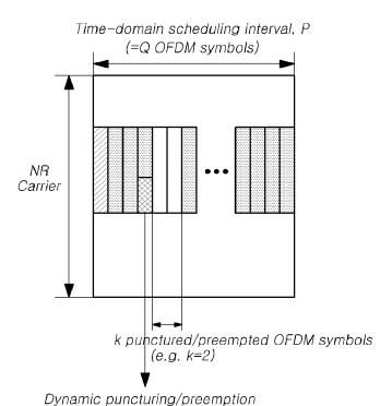
Case a. in-band dynamic puncturing/preemption indication channel transmission
