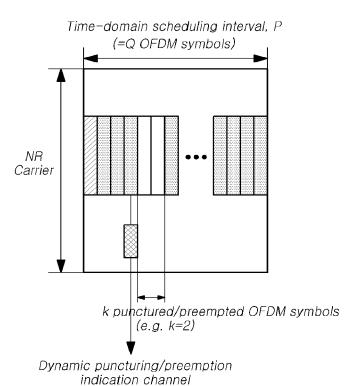
Case b. out-band dynamic puncturing/preemption indication channel transmission
