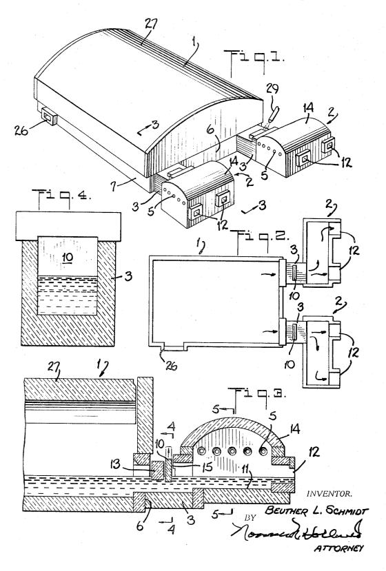
GLASS FURNACE WITH TWO SEPARATE THROAT PASSAGES
