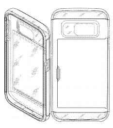
FIG. 15 is a front perspective view of the rear compartment cover component of the case shown in isolation for clarity of disclosure:
