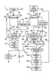
60% and more preferred at least 90% of a total amount of alkaline agent supplied to the cleaning system is supplied to the second scrubber process loop.
