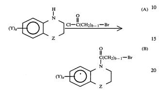
acyl chloride with an  $\omega$ -bromo group. However, any suitable halo leaving group can be used in either position, for example, the acyl bromides or  $\omega$ -chlorides or iodides are also appropriate.
