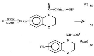
In carrying out this sequence, a sodium alkoxide of formula NaOR<sup>1</sup> is added to a solution of the compound 65 of formula B in the corresponding alcohol. The mixture is then kept at 50° to 150°, preferably reflux temperature for 2 to 24 hours, preferably 8 hours. The compound of
