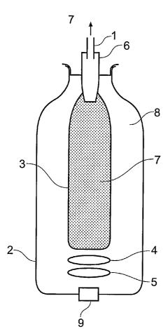
(57) Abstract: This invention relates to devices and systems for the pressurised dispensing of fluid, in particular from a container provided with a valve or tap (6). The propellant is generated by a chemical reaction.
