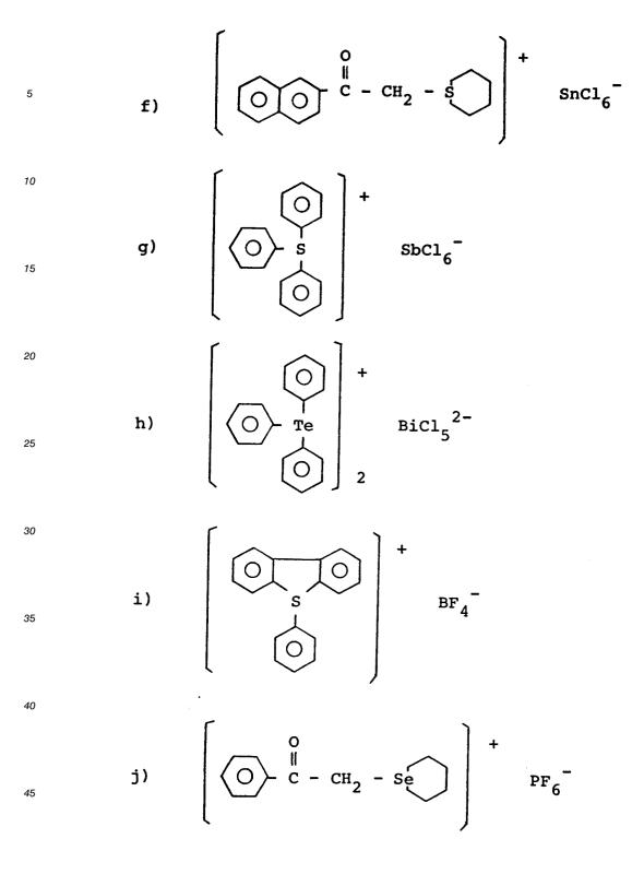
and photosensitive aromatic onium salts of the elements belonging to the group Va as shown below:
