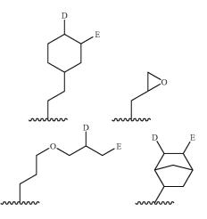
where D and E independently are hydrogen, hydroxy-, acetoxy- groups, alkylalkoxy- or alkylacetoxy- groups or D and E can form a cyclic epoxide, the molar fractions x, y and z independently represent a value from 0 to about 0.8 and the sum of x, y and z equals 1; or
