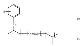
where  $R_3$  is a linear, branched, or cyclic alkylene group of 1 to about 10 carbons, G is hydrogen, hydroxy-, acetoxy-, methoxy-, ethoxy- or other alkoxy-, halogen, ester, carboxy- or a carboxamido-group, J is alkyl, alkoxy-, or up to about 6 carbon atom carboalkoxy or alkoxycarbonyl esters, lactone or anhydride moieties, the molar fractions x, y and z independently are from 0 to about 0.5 and the sum of x, y and z equals 1, and the amide group is an organic amidic group: 25
