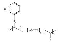
where  $R_3$  is a linear, branched, or cyclic alkylene group of 1 to about 10 carbons, G is hydrogen, hydroxy-, acetoxy-, meth-
