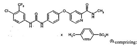
adding thionyl chloride to 2-picolinic acid in a solvent inert toward thionyl chloride without using dimethylformamide and reacting to give a compound of the formula (III)
