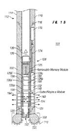
(57) Abstract: A method of estimating a property of interest downhole according to one aspect of the disclosure may include continuously receiving a core drilled from a formation into an open end of a chamber while removing the core distal from the open end of the chamber; obtaining a measurement relating to property of interest of the core using at least one sensor; and estimating the property of interest of the core using the obtained measurement.
