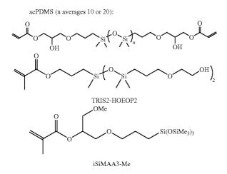
The results, shown in Table 4, show that SiGMA, acPDMS (where n=10 and 20) and mPDMS-OH more readily incorporate into a blend of a diluent, another silicone containing monomer, a hydrophilic monomer, and an high molecular weight polymer (PVP) than alternative silicone-containing monomers. Thus, compatibilizing silicone containing monomers having a compatibility index of greater than about 0.5 are useful for compatibilizing high molecular weight hydrophilic polymers like PVP.
