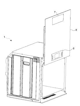
(57) Abstract: The present invention relates to a household appliance (1) that allows the panel (3) to be viewed by means of a door (8) when the front of the body (2) is in the open or closed position.
