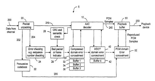
(57) Abstract: Audio data from a channel (200) is AAC decoded (10) and the data is checked for errors (24). If a bad packet or frame is detected (28), then the signal is processed to conceal the error (30, 40, 52).
