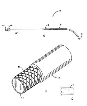
(57) Abstract: The present invention is a guide catheter and a method of making the guide catheter. The invention includes a catheter having an inner layer, a support element associated with the inner layer, and an outer layer external to the support element. The invention further includes a cutting apparatus used in the method of making the guide catheter.
