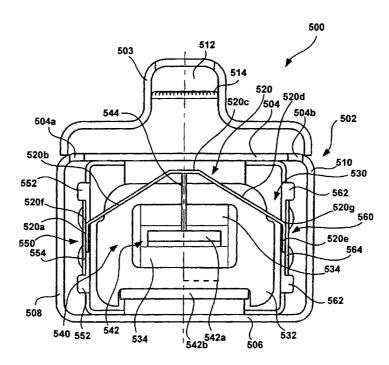
(57) Abstract: A receiver assembly includes a first diaphragm assembly having a diaphragm, and a second diaphragm assembly having a diaphragm. A linkage assembly is coupled to an armature of the receiver. The linkage assembly is also coupled to the first diaphragm assembly and to the second diaphragm assembly.
